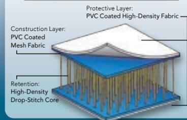
Each kayak is constructed of High Pressure Drop-Stitch material for a solid hard-boat like stiffness.
