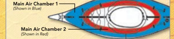
Our unique design divides the main inflation chamber into two separate air chambers that encompass the entire kayak. This provides optimum safety when out on the water.
