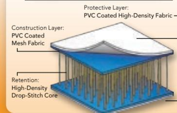
Each SUP is constructed of High Pressure Drop-Stitch material for a solid hard-board like stiffness.
