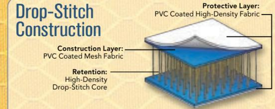
Each SUP is constructed of High Pressure Drop-Stitch material with a double layer of PVC Tarpaulin for a solid hard-board like stiffness.
