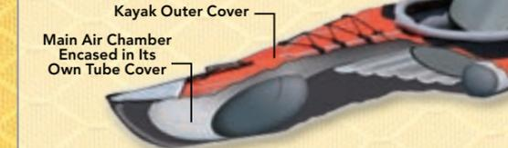
Unlike many inflatable kayaks, our kayaks are developed with multiple layers of material for maximum durability.
