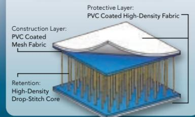
Each kayak is constructed of High Pressure Drop-Stitch material for a solid hard-boat like stiffness.
